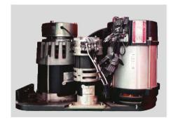
German Schabmuller Drive motor and steering motor.
